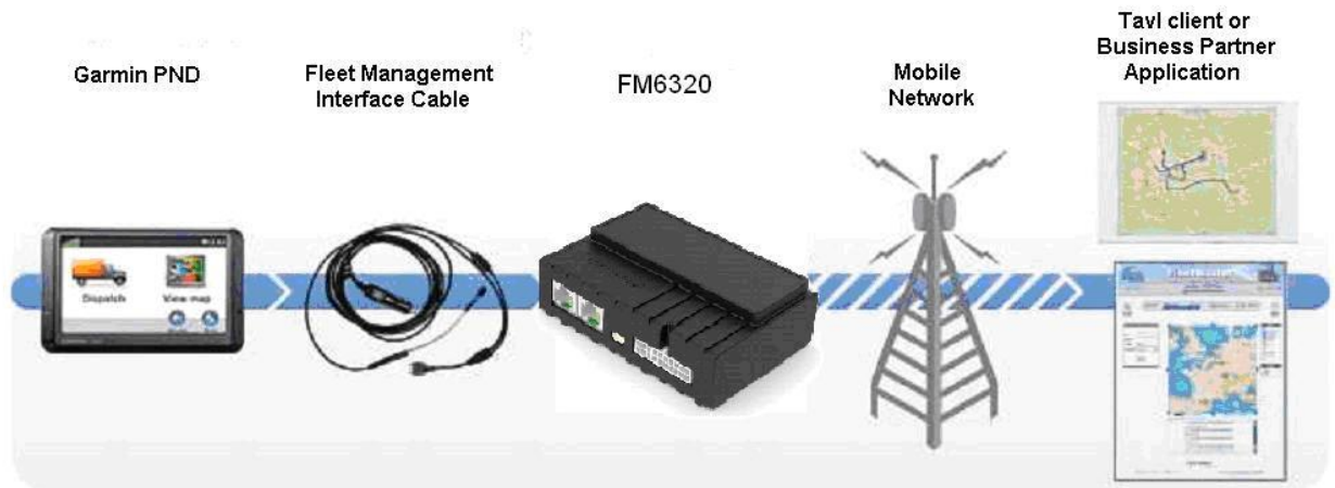
Figure 115 FMB630 +Garmin operational scheme
